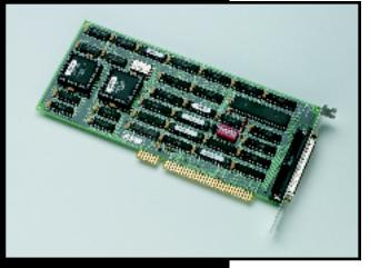
• 24 TTL/CMOS digital I/O Lines
